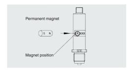
To correct the zero point, hold a permanent magnet (e.g. pin board magnet) at the position marked on the pressure transmitter (the encircled letter) approximately 30–150 seconds after the voltage supply has been switched on.
