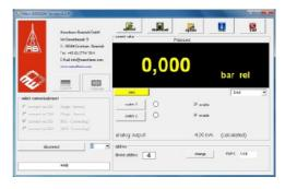
When switching between different transmitters (measuring points) in bus operation, the "zero" button is highlighted yellow if the "Offset" register is not set to "0", which means that a previous zero setting is still set. This indicates that no new taring of the measuring chain was performed.
