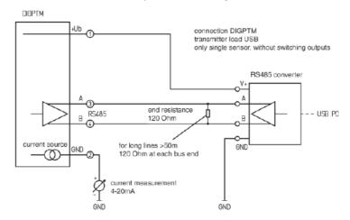
During bus operation of several transmitters, the provided current of the PC USB port is not sufficient. An external current supply is necessary.
