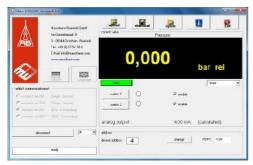
With taring, the current measured value is added to the register "Offset" and is thus thereafter always subtracted (see point "output options"). Thus, it is possible to measure "gauge pressures" even with absolute pressure transmitters and to suppress fluctuations of the air pressure or the geographical installation altitude.
