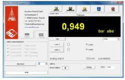
The button "zero" serves for the zero setting of the atmospherically vented transmitter before starting the gauge pressure measurement (the addition "abs" in the display disappears); the display is set to "0", the "zero" button is highlighted green.
