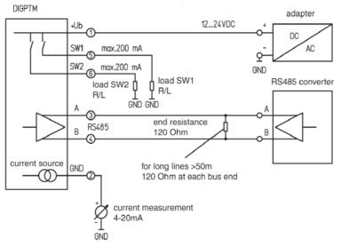
external connection DIGPTM with switching outputs
