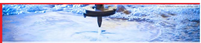
The functional principle of water jet cutting and high-pressure cleaning is basically the same. Water is pumped via a line to a nozzle, to then be jetted under varyingly high pressure. But depending on the application, the requirements increase. The higher the pressure, the more complex the technology. In order to control pressures up to 4000 bar, the pressure gauges also have to meet high demands.
